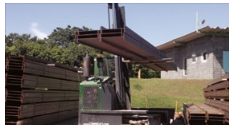
Empilhadeiras Side Loader. Side loading forklifts.
