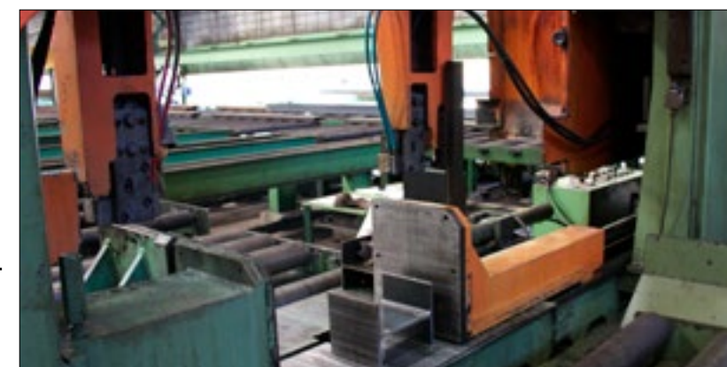
Serra para cortes retos. Bandsaw for vertical cutting.
